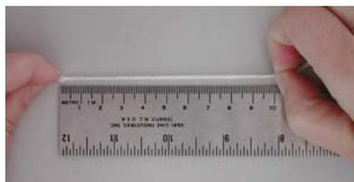
After measuring a root, placing the string next to a ruler to calculate the actual root length.
